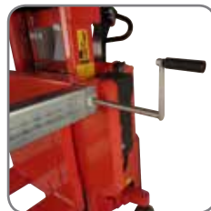
Adjustable box holders: The width is adjusted by a handle, so that the width fits the requested box width (between 800 mm and 1200 mm).
