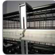
Box holders with or without clamps (optional extras) can be fitted. Clamps are recommended when tilting more than 60°.
