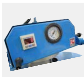
Vacuum monitor , prevents lifting if vacuum level should not be sufficient. Adjustable for the goods that is to be handled.
